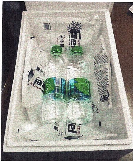
Figure 1. The packing arrangement in the expanded polystyrene container. T_{\text{water}} was monitored by placing a type K thermocouple directly inside the water, through a small hole in one of the bottles.
